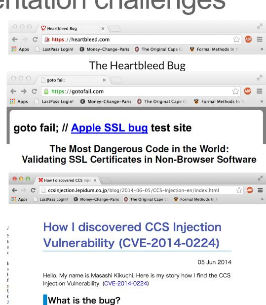
The problem is that OpenSSL accepts ChangeCipherSpec (CCS) inappropriately during a handshake. This bug has existed since the
